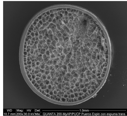
Fig. 2 – Scanning electron microscopy (SEM) image of a cross-sectional view of a porcupine quill sample showing the interior foam core surrounded by an outer shell.
